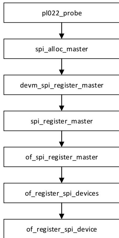
Parses SPI controller node of the DTS file to obtain the relevant hardware information, initialize the SPI controller, match the compatible attributes in DTS file, register the SPI controller, register the SPI device to the bus.
