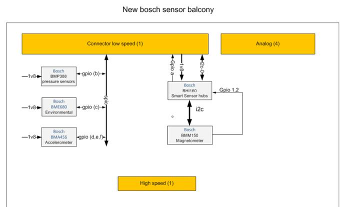
All sensors are activated from the 1.8v voltage and controlled by spi-0, i2c-0 and 6 gpio lines (gpio a,b,c,d,e,f).
